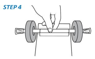
Cut two 3-inch pieces from the plastic straw. (Note: Save the final piece of straw for the Lesson 2 experiment.) Flip the car over and tape the straw pieces along the guidelines on the bottom of the car.
